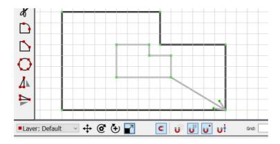
The external dimensions of the selected objects are displayed on the top bar of the program and can be modified manually (by entering the X Y dimension values from the keyboard).
