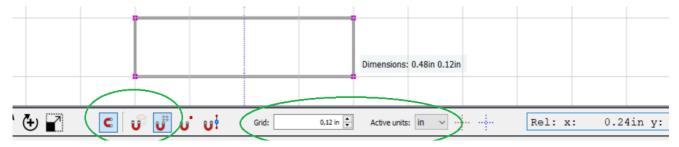
It is also possible to enable the cursor to snap (while drawing) to points on an object and to snap to the centre of a segment.
