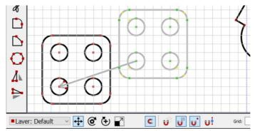
The position of selected objects (their geometric centre) in relation to the selected datum is displayed on the top bar of the software and can be modified manually (by entering XY values from the keyboard).
