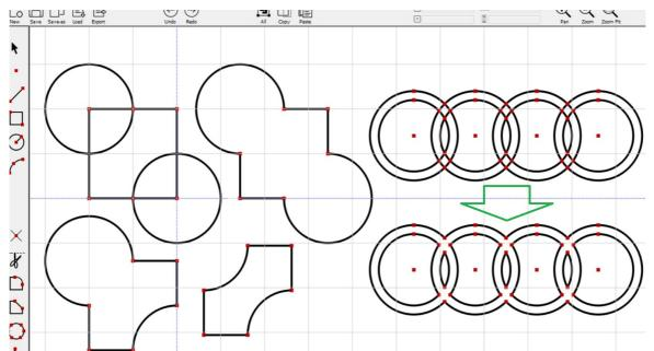
The tool works on pre-selected objects or, after selecting the tool, you can click on the object to be sectioned with collision objects.
