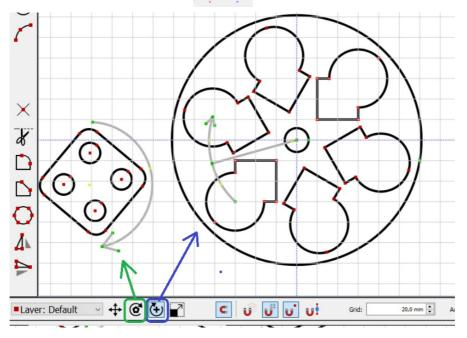
By default the resolution of rotation is set to 2.5 degrees, Holding down the [Ctrl] key it is possible to rotate objects freely.
