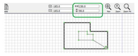
Scaling is done by proportionally changing the distance between control points. Due to this specificity, the algorithms do not work properly for arcs and circles.
